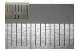
Surface texture can be seen and might disturb accurate imaging
