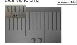
Surface texture is no longer visible, making it possible to read the printed text more clearly
